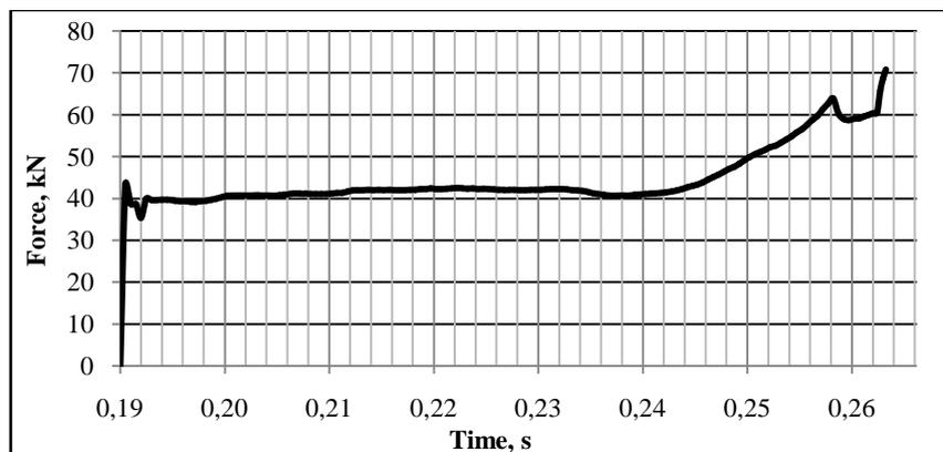
**Fig. 8. Forming force versus time in the third stage of the flanging process**
