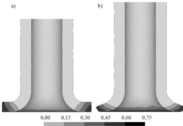
**Fig. 4. Changes in the workpiece shape and the damage function distribution (calculated according to the Cockcroft-Latham criterion) in the second stage of the flanging process: a) flanging with a movable sleeve, b) flanging with an internal sleeve [source: own study]**
