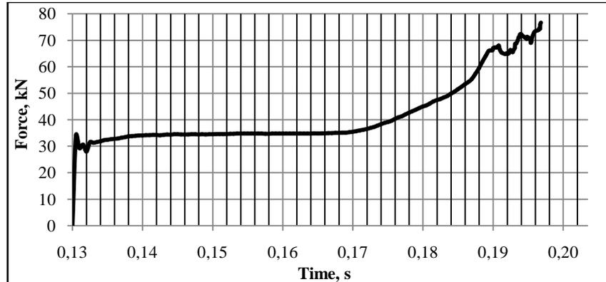
**Fig. 7. Forming force versus time in the second stage of the flanging process**
