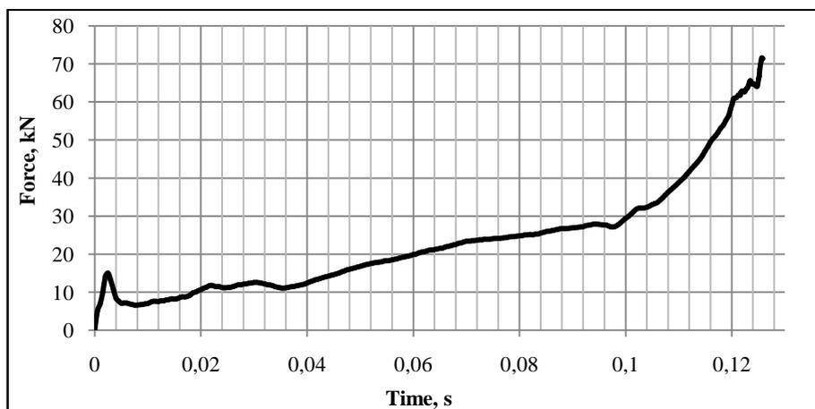
**Fig. 6. Forming force versus time in the first stage of the flanging process**
