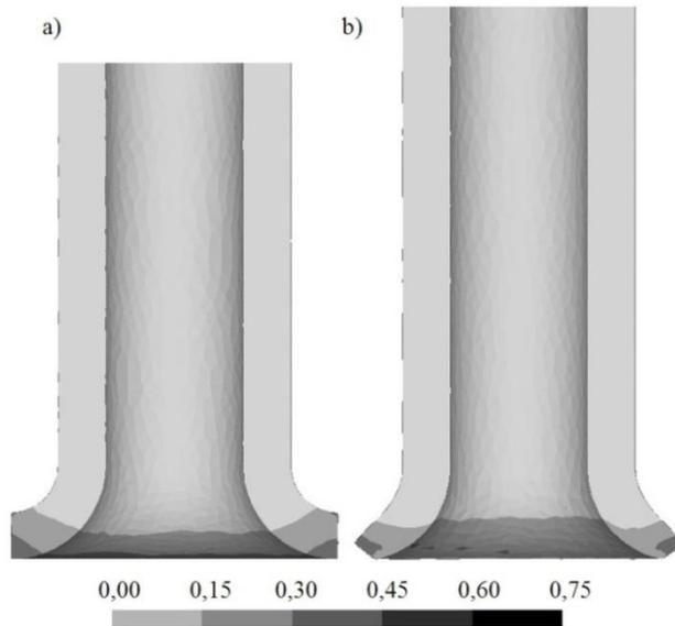
**Fig. 3. Changes in the workpiece shape and the damage function distribution (calculated according to the Cockcroft-Latham criterion) in the first stage of the flanging process: a) flanging with a movable sleeve, b) flanging with an internal sleeve [source: own study]**
