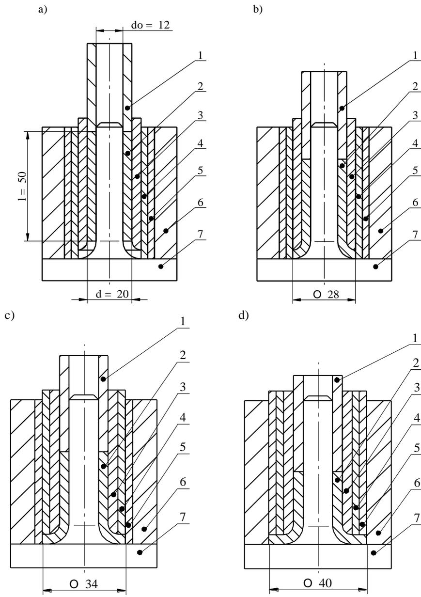
**Fig. 2. Design of the flanging process, where: 1 – punch, 2 – workpiece, 3 – internal sleeve, 4 – first movable sleeve, 5 – second movable sleeve, 6 – external sleeve, 7 – mandrel, a) initial stage of flanging, b) first stage of flanging, c) second stage of flanging, d) third stage of flanging [source: own study]**
