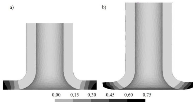
**Fig. 5. Changes in the workpiece shape and the damage function distribution (calculated according to the Cockcroft-Latham criterion) in the third stage of the flanging process: a) flanging with a movable sleeve, b) flanging with an internal sleeve [source: own study]**
