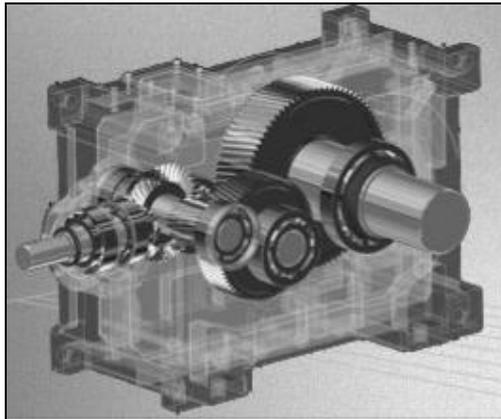
**Fig. 2. The 3D model of helical-bevel reducer BH [32]**
