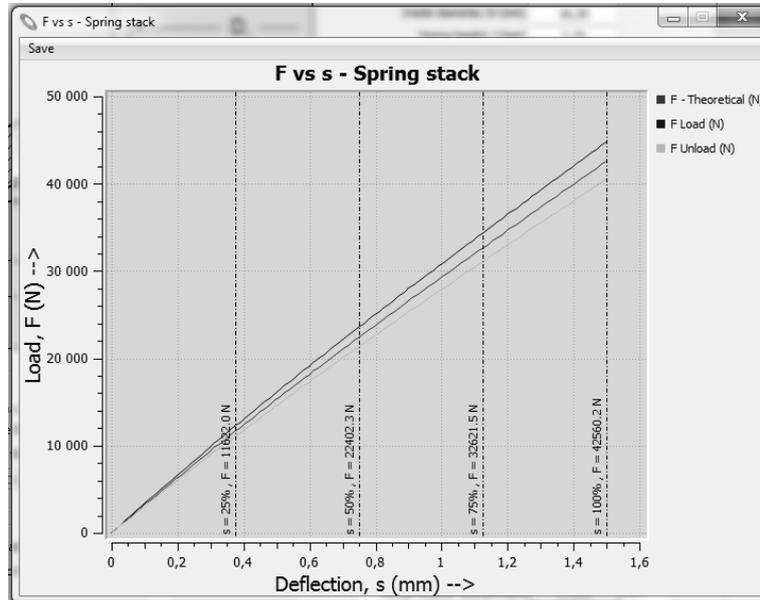
**Fig. 6. Deflection characteristics of disk spring package matched with catchers in Disk Spring Solver application [source: own study]**
