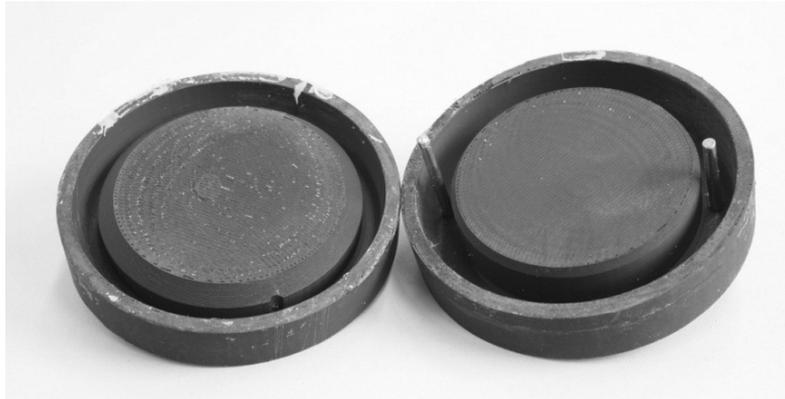
**Fig. 4. Halves of the casting mold produced using FDM technology [source: own study]**
