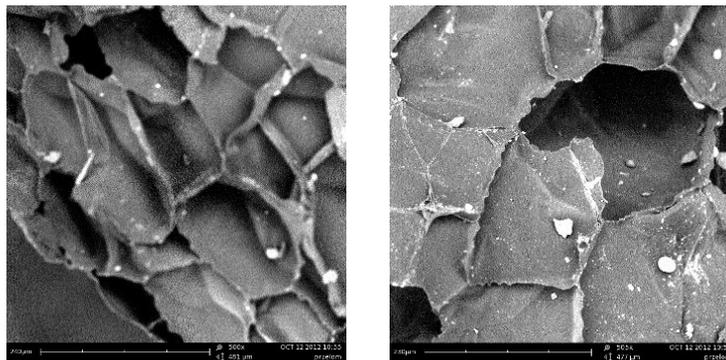
**Fig. 1. SEM image of section structure – polypropylene foam [source: own study]**
