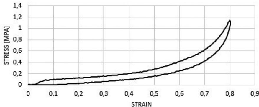
Fig. 2. Example experimentally determined hysteresis loop [source: own study]
