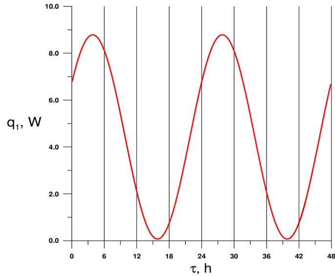
**Fig. 10. Periodically heat flux flow signal on the wall –  $q_1$  [source: own study]**
