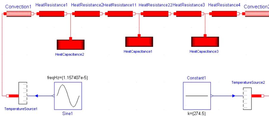
**Fig. 7. Block schema using electrical analogue [source: own study]**
