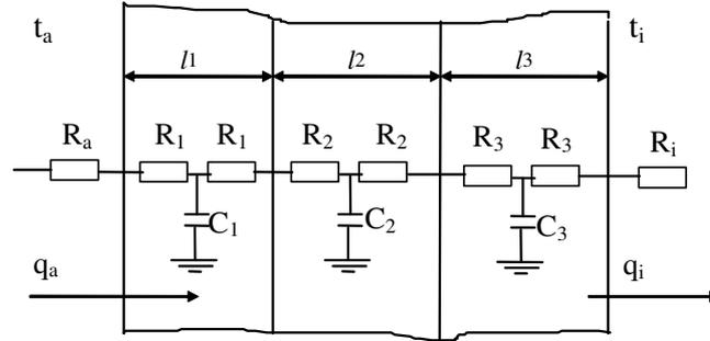
**Fig. 5. Model of wall composed of three layers in electrical analogy [source: own study]**
