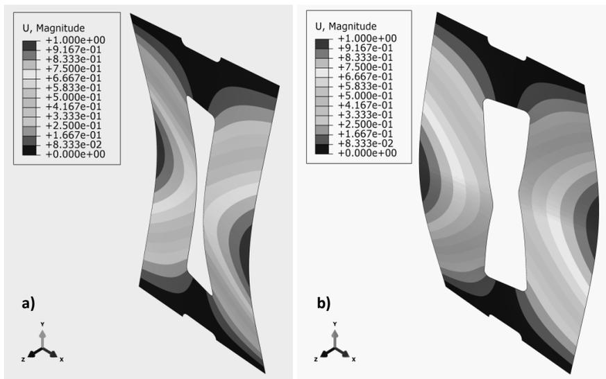
Fig. 3. Examples of buckling form plates with cut-out in ABAQUS program
