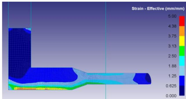
Fig. 8. Strain diagram for E.R.: 4 die angle: 20 [source: own study]
