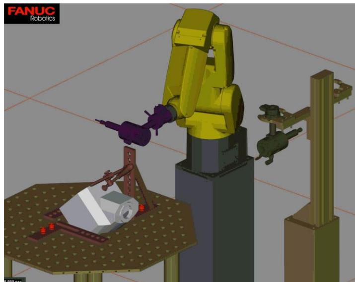
**Fig. 5. Designed robotic cell for automation of deburring technology (Roboguide HandlingPRO) [9]**
