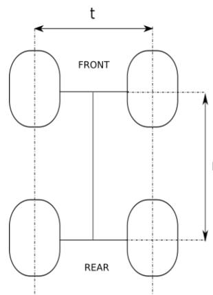
**Fig. 1. Track and wheelbase measurement [source: own study]**
