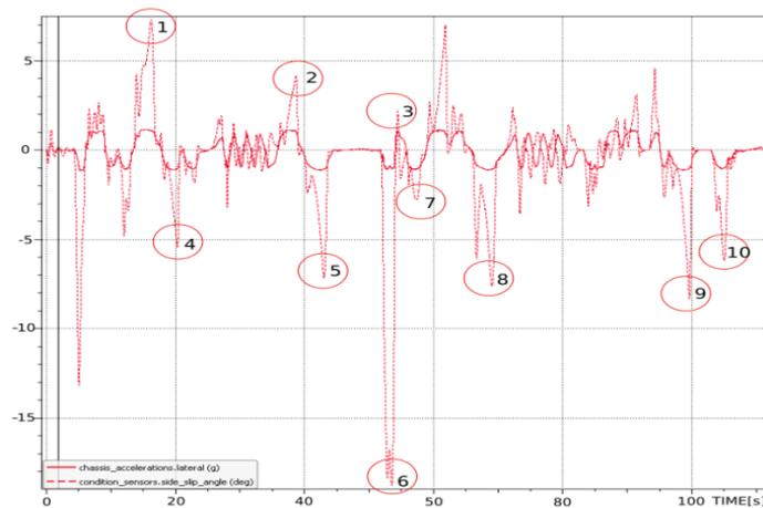
**Fig. 8. Side-slip angle in degrees (dotted line) and chassis lateral acceleration in G rate (solid line) of a car with wider front track [source: own study]**
