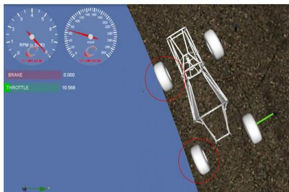
**Fig. 5. Preview of collocation in the sample corner, car with both tracks equal to 1100 mm [source: own study]**
