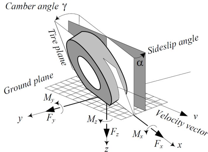
**Fig. 2. SAE tire coordinate system [8]**
