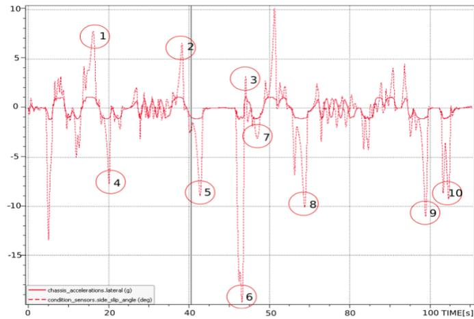
**Fig. 10.** Side-slip angle in degrees (dotted line) and chassis lateral acceleration in G rate (solid line) of a car with both tracks set equal to 1200 mm [source: own study]
