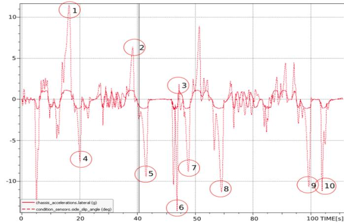
**Fig. 9.** Side-slip angle in degrees (dotted line) and chassis lateral acceleration in G rate (solid line) of a car with both tracks set equal to 1100 mm [source: own study]
