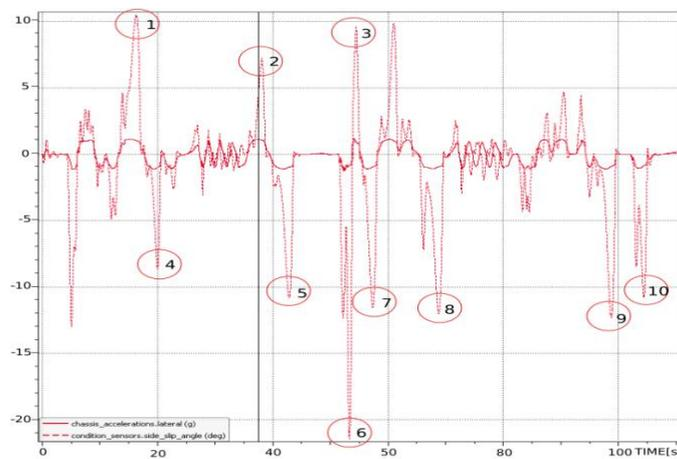
**Fig. 7. Side-slip angle in degrees (dotted line) and chassis lateral acceleration in G rate (solid line) of a car with wider rear track [source: own study]**
