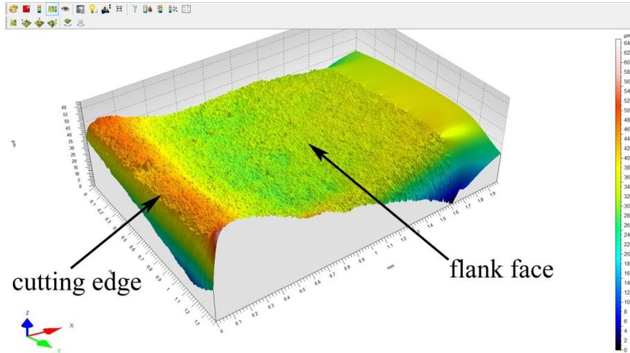
**Fig. 4. Flank face topography of insert no. 1 [source: own study]**
