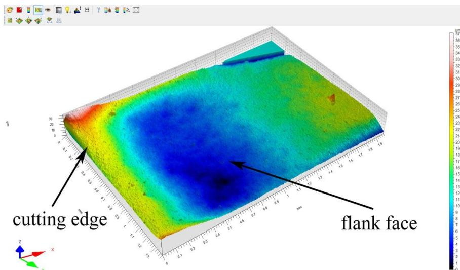
**Fig. 5. Flank face topography of insert no. 2 [source: own study]**
