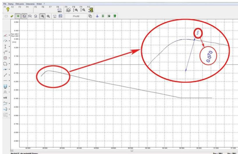
Fig. 3. Measurement of edge rounding [source: own study]
