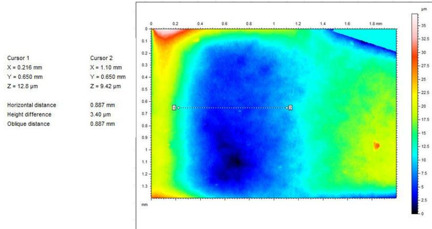
**Fig. 6. Length measurement on the 2D map [source: own study]**
