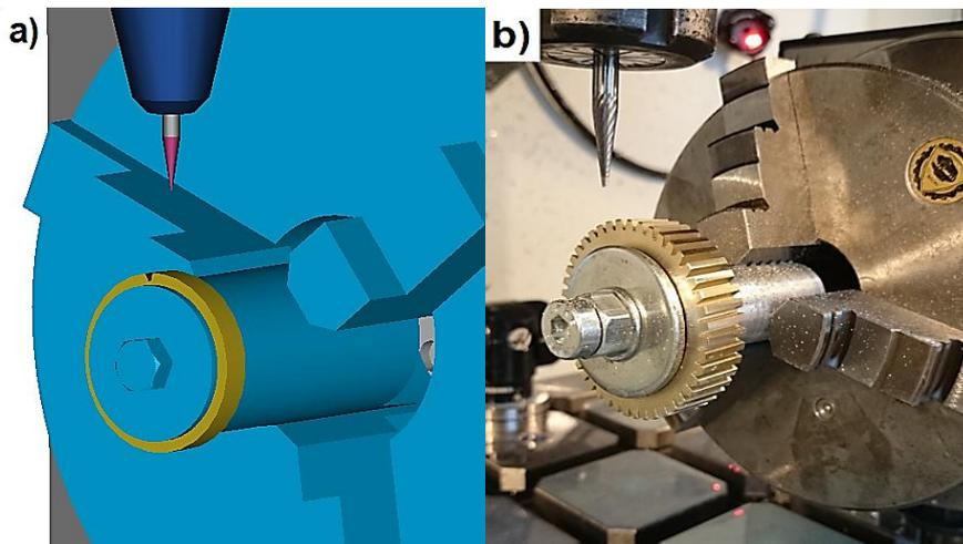
**Fig. 7. Simplistic tooth space machining: a) CAM simulation, b) machining on machine [source: own study]**
