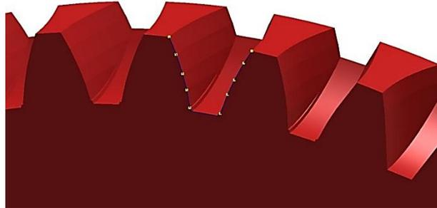
**Fig. 3. Approximate shape of tooth space with characteristic point [source: own study]**
