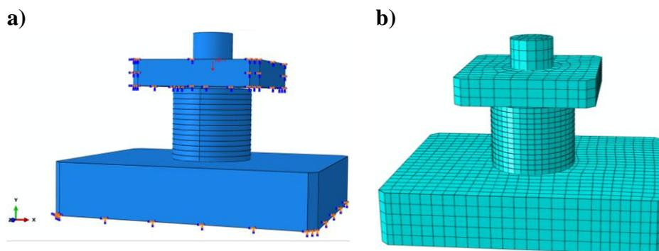
**Fig. 3. a) Boundary conditions of the system , b) FEM mesh – total numbers of nodes: 10292; total numbers of elements: 5862, 5862 linear hexahedral elements of type C3D8R (own study)**
