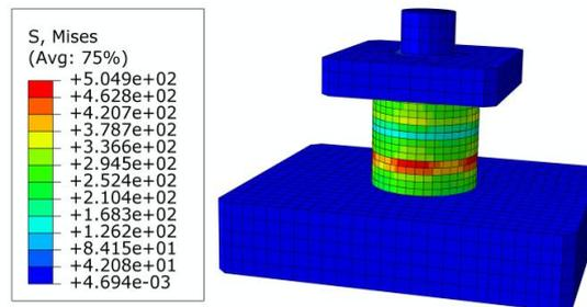
Fig. 4. Numerical results of stresses: a) package 14V under load of 21kN, b) package 7V7 under load of 38kN, c) package 4V5X5 under load of 38kN (own study)
