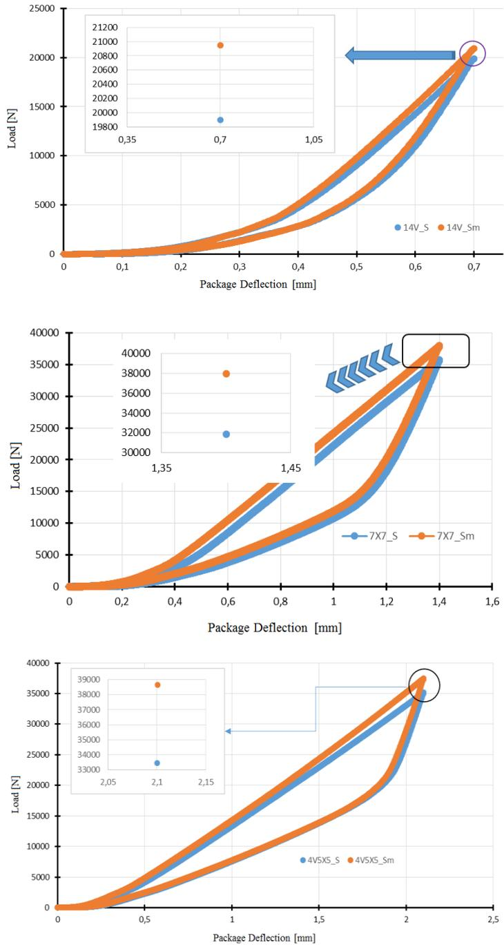
**Fig. 6. Experimental results of spring package deflection (own study)**
