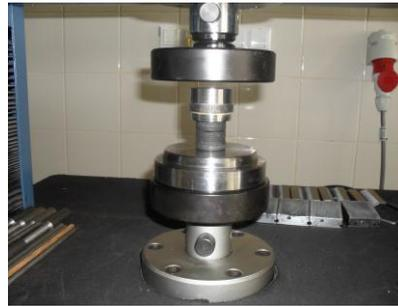
**Fig. 2. 4V5X5 disk spring package configuration to be tested using HT-2402 machine (own study)**
