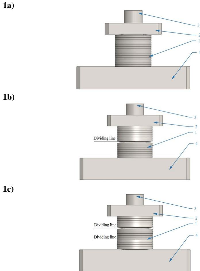
**Fig. 1. Models of disk spring packages designed in Solid Works: 1 – disk spring package, 2 – pusher, 3 – guiding bolt, 4 – base, a) configuration 14V, b) configuration 7V7, c) own study**
