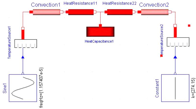
**Fig. 9. Ideal model passage of heat through the baffle using an analogy to Ohm's law (own study)**
