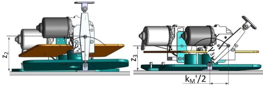
Fig. 4. Second and third stage of tilting simulation (own study)
