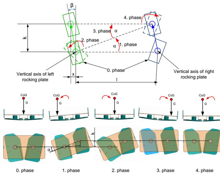
Fig. 2. Phases of movement to forward (own study)
