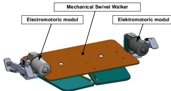
Fig. 1. Swivel walker with electromotoric modules (own study)
