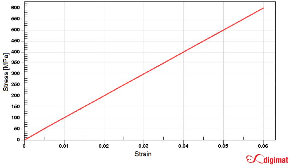
**Fig. 4. Stress-strain characteristic for wood fiber (elastic range)**
