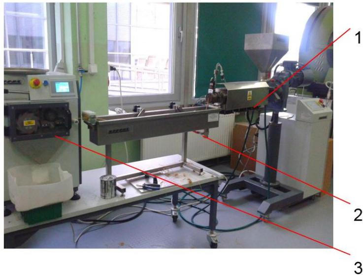
**Fig. 2. Manufacturing of WPC composites: 1 – Zamak EPH-25 extruder, 2 – cooling bath, 3 – granulator**
