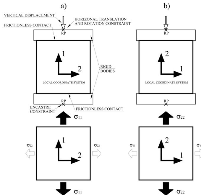
**Fig. 5. Compression test with different local coordinate systems orientation:
