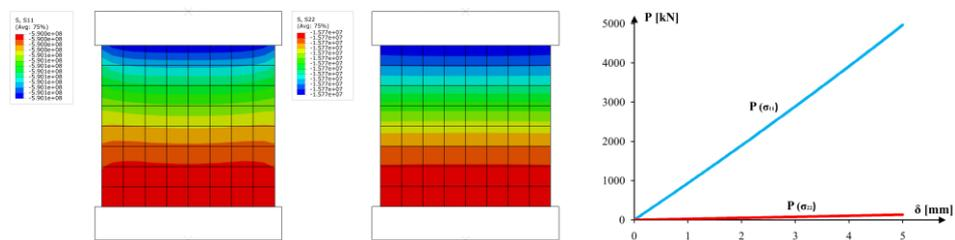
Fig. 16. CPS8 elements displacements,  $\sigma_{11}$ ,  $\sigma_{22}$  stresses distribution and  $P$ - $\delta$  relation
