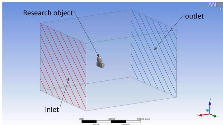
**Fig. 2. The research object in the research area with the boundary conditions – isometric projection**
