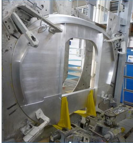
Fig. 7. The finished frame mounted in the device used for checking the aircraft frames
