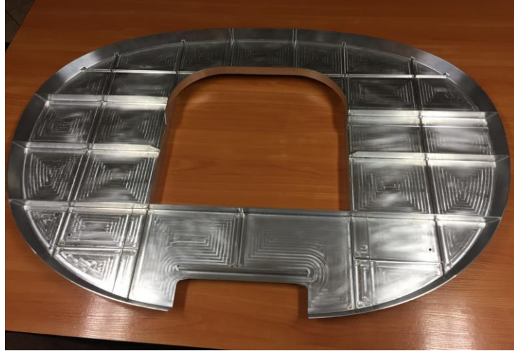
Fig. 3. The finished frame after mechanical machining (shaping)
