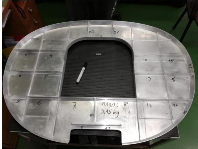
Fig. 6. The measurement points layout (the part after finishing)
