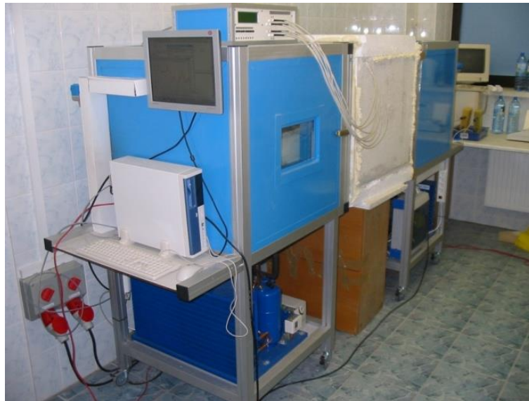
Fig. 2. Registering positions laboratory with two temperature chambers and the test material in the middle
