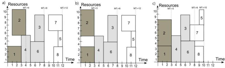
**Fig. 6. Schedules: a) backward schedule generated for activity list  $\{1, 5, 2, 3, 4, 6, 7, 8\}$  using initial completion dates for stages:  $MT_1 = 4, MT_2 = 8, MT_3 = 12$ , b) schedule determined as a result of optimization of the completion date for the first stage:  $MT_1 = 3, MT_2 = 8, MT_3 = 12$ , c) Schedule determined as a result of optimization of completion dates for three project stages:  $MT_1 = 3, MT_2 = 8, MT_3 = 10$**
