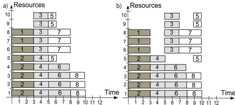
**Fig. 5. Schedules: a) schedule generated for activity list {1, 2, 3, 4, 5, 6, 7, 8} with resource allocation determined with the use of the RALS procedure, b) schedule corrected with the use of the right-shift procedure**
