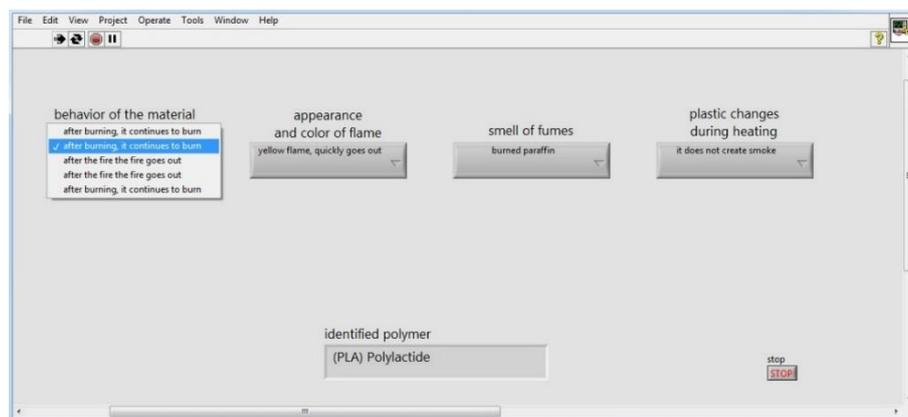
**Fig. 3. Program view in the form of a user panel**
