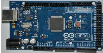
**Fig. 1. Arduino Mega 2560 board**
