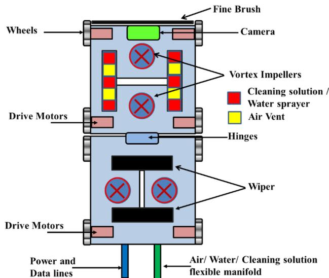
Fig. 7. The proposed model of the Robot
