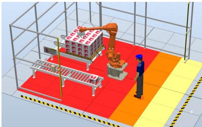
**Fig. 2. Human operator in the 2<sup>nd</sup> safety zone**
