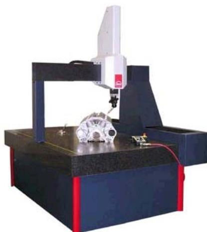
Fig. 3. MORA – CNC Measurement and Digitization Machine
