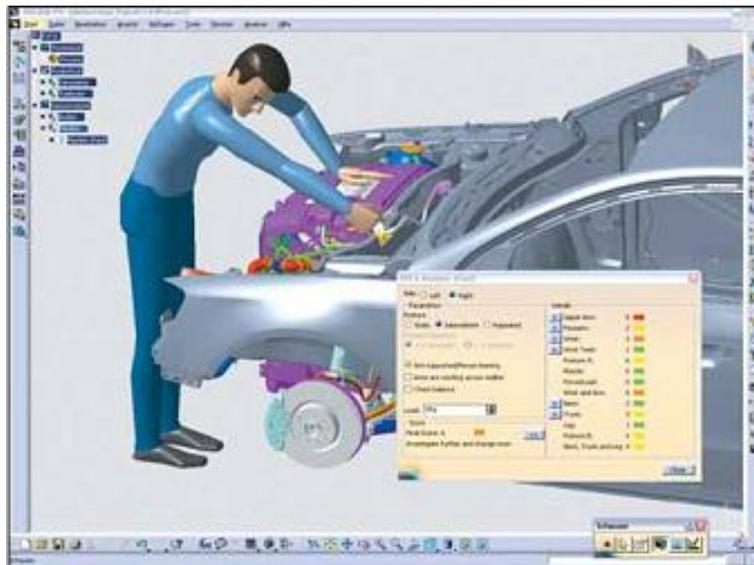
Fig. 2. Digital assembly with Delmia V5 DPM Assembly in Volkswagen AG
