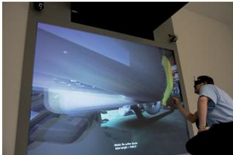
Fig. 1. Virtual Assembling at an L-shaped Display
