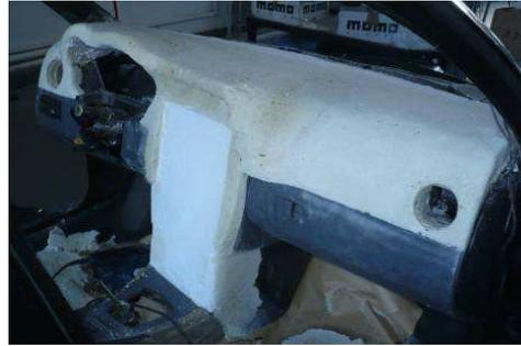
Fig. 10. Dashboard fabrication
