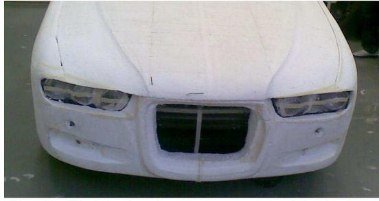
Fig. 21. Finished polystyrene model of the bumper
