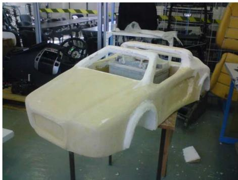
Fig. 7. Mockup fabrication (scale 1:4)
