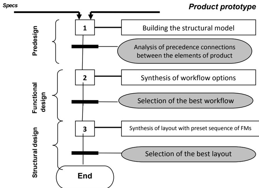
Fig. 7. Algorithm for the directed synthesis of technological equipment
