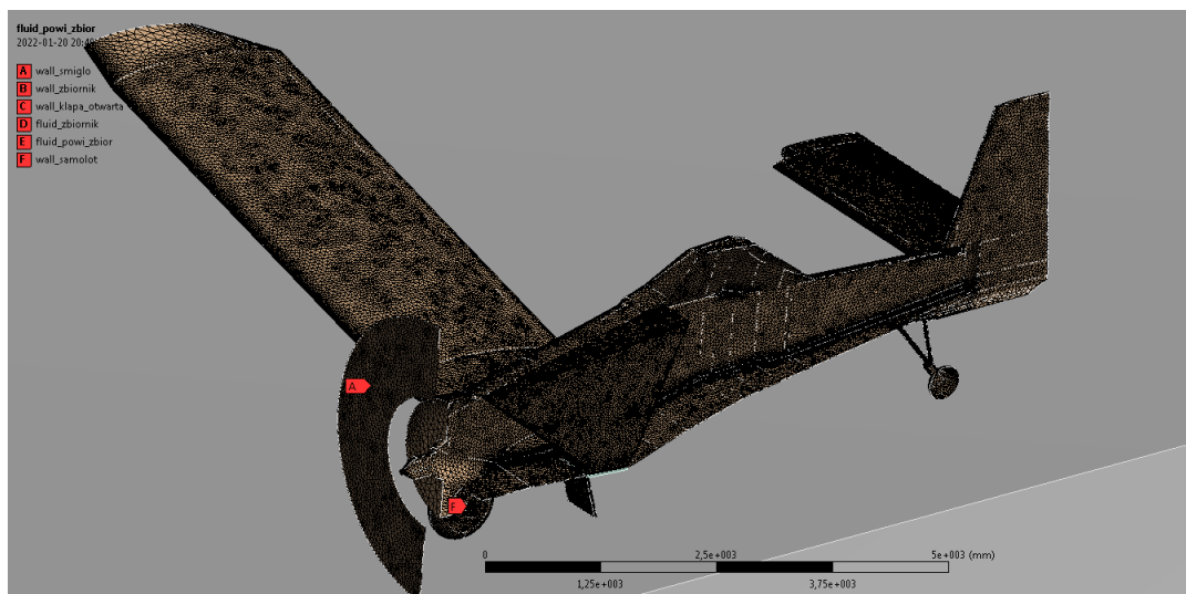
Fig. 5. Computational mesh on the surface of the examined object
